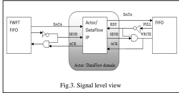
Fig.3. Signal level view
