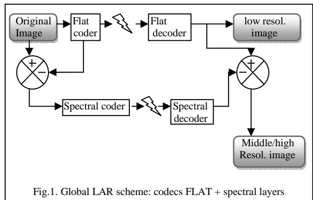
Fig.1. Global LAR scheme: codecs FLAT + spectral layers
