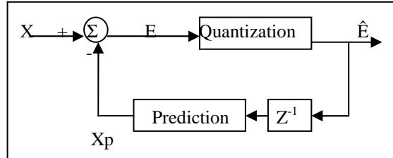
Fig. 4. The DPCM principle
