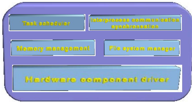
Figure 2: Embedded OS architecture
