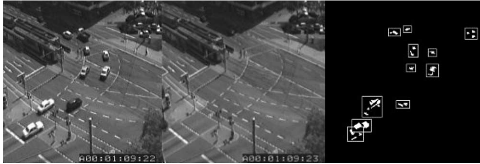
Fig. 4. Smart camera executing. Left, video from the camera; center, background detection; right, moving objects detection.
