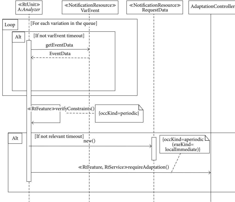
FIGURE 6: Behavioral view of the RTE Analyzer pattern.
