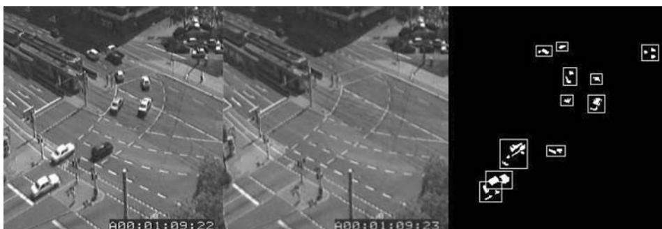
Figure 10. OMD motion detection example. Video/background detection/moving object detection.
